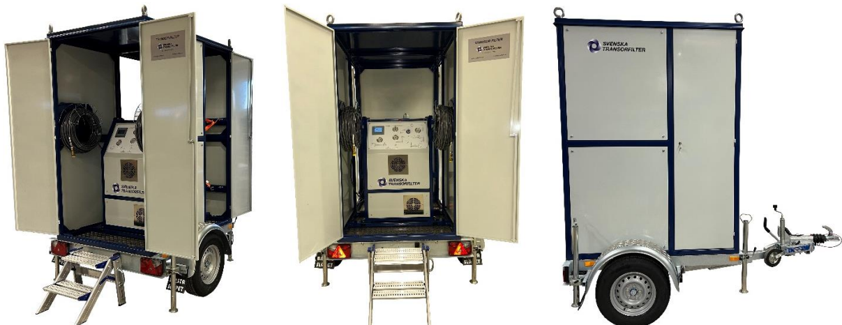
FV2C-CW mobile road-worthy trailer version.
