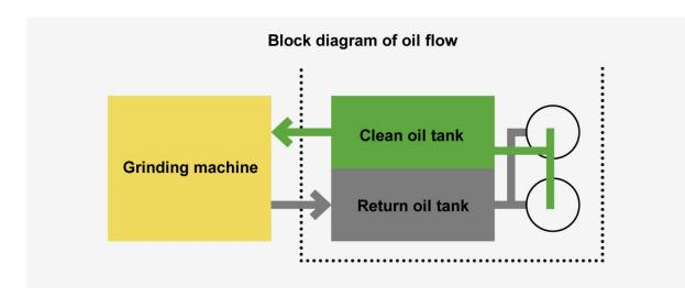
Size and amount of filter vessels depends on application. Filter may be prepared for connection of multiple machines in the future.
